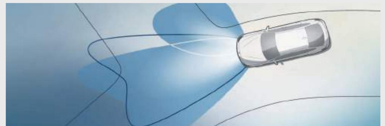
With the **fully adaptive LED headlights**, not only does the outer light move with the steering but also the 4 source LED (low and high beam) including DRL's which distinguishes the look of the BMW X3 both at night and during daytime.
