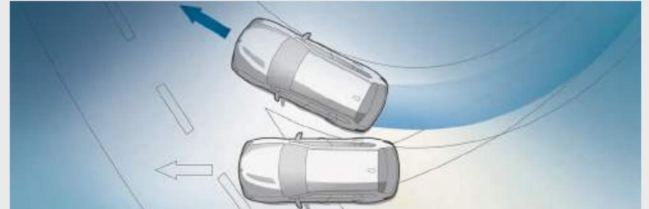
**Dynamic Stability Control (DSC)** permanently assesses the vehicle's movements and stabilises it using engine and braking regulation when unstable driving conditions are detected. Additional features of DSC are, for example, brake drying, braking readiness or the Hill-Start assistant, which holds the vehicle briefly in place when starting on inclines to prevent it from rolling backwards.
