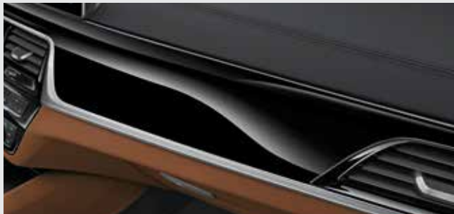
The instrument panel in Sensatec lends the interior of the vehicle a highly exclusive atmosphere. The artificial leather is applied directly to a semi-rigid foams and features an impressively soft surface.
