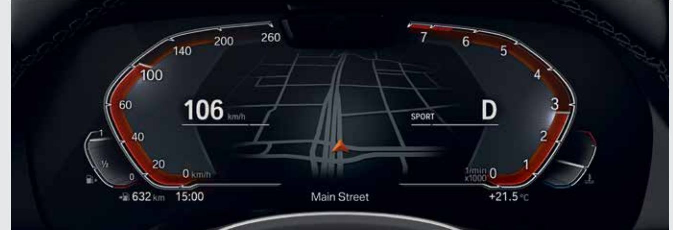
The newly designed Instrument Display with Black Panel technology and a screen diagonal of 31.2 cm (12.3") provides a highly impressive visualisation of the driving experience. The different modes and their specific displays – each of which has its own colour scheme and graphic style – can be displayed in the instrument cluster.
