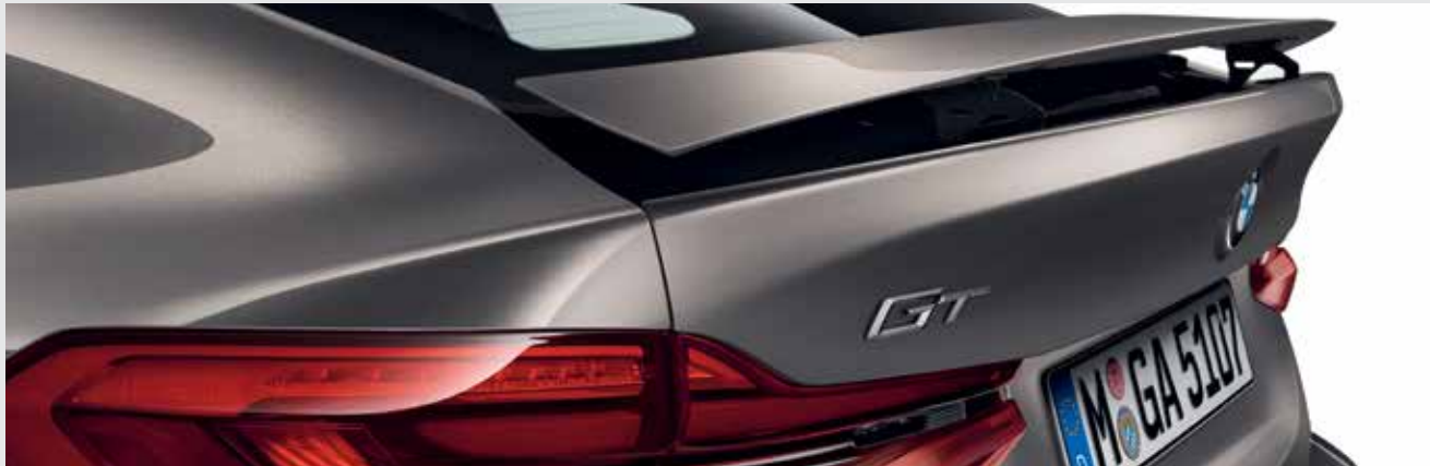
The Active Rear Spoiler automatically extends at a speed of over 110 km/h and retracts once the speed returns to 70 km/h in order to improve stability.
