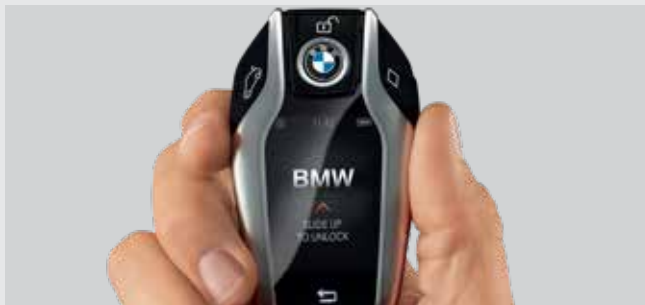
The BMW Display Key shows various information about the vehicle's status and allows selected functions to be controlled with an integrated touch display.
