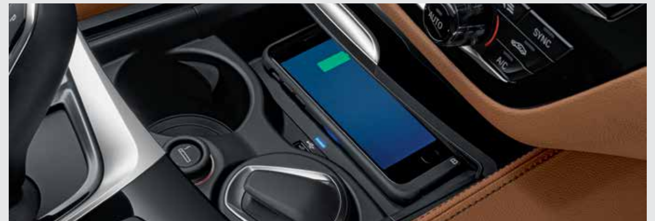
Telephony with wireless charging 1 includes a wireless charging dock and additional USB ports. A roof aerial connection improves mobile reception. Two mobile telephones and an audio player can be connected simultaneously via Bluetooth.
